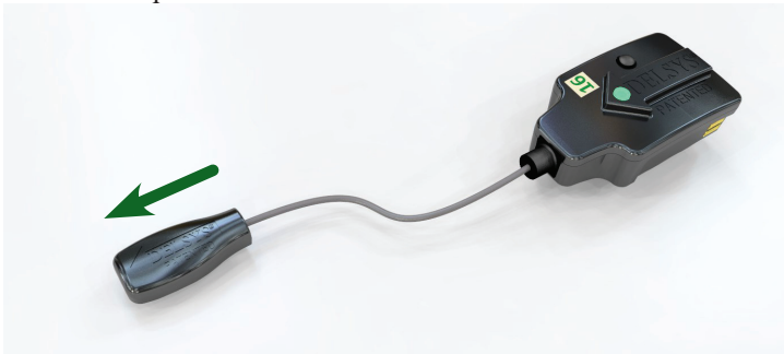
Figure 7. The MiniHead sensor top is marked with an arrow which must be placed parallel to the muscle fiber direction in order to properly detect an EMG Signal.
