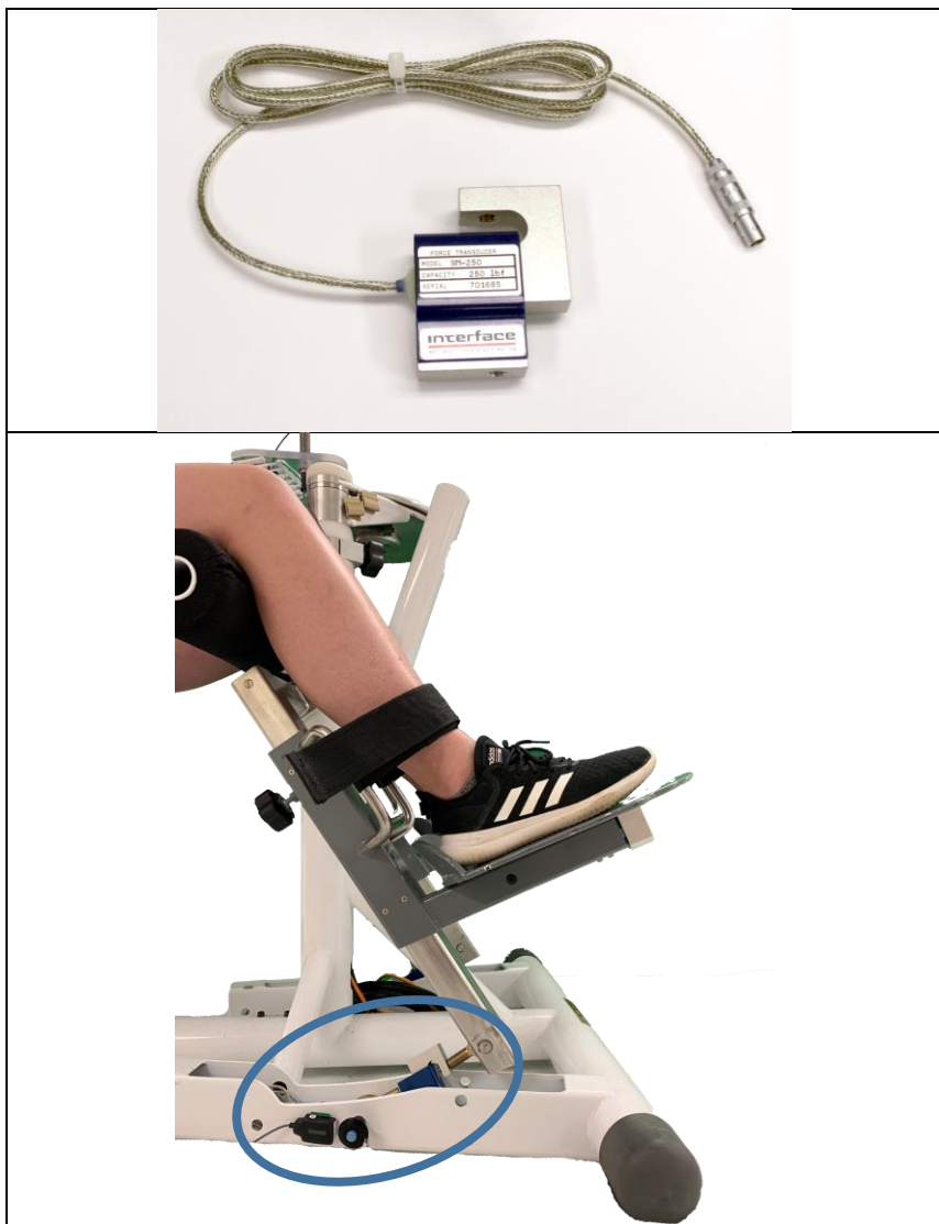
Figure 3: Load Cell transducer (top) affixed to an isometric setup (bottom).
