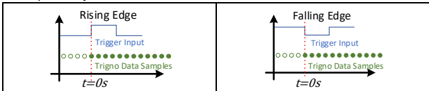
Figure 17: Start Trigger Input data sample timing for rising or falling signal edges.
