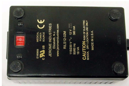
Figure 11. Underside of Power Supply showing the red Line Voltage Selector switch.
