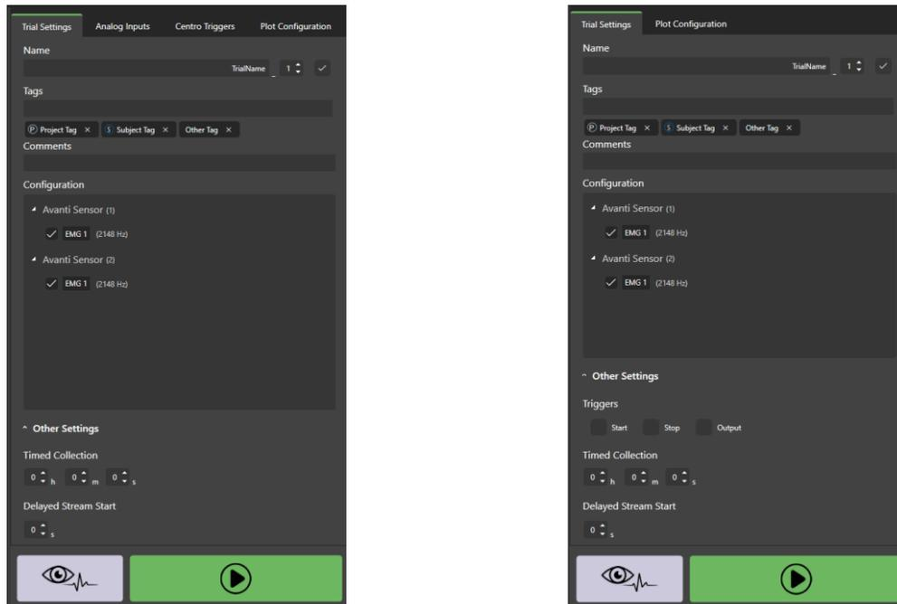
Figure 10: a) Trial Settings tab with Trigno Centro, b) Trial Settings tab with Trigno Base
