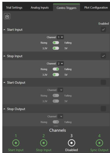
Figure 13: Trigno Centro Triggers tab
