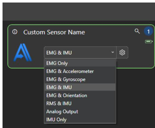
Figure 5: Quick sensor mode selection
