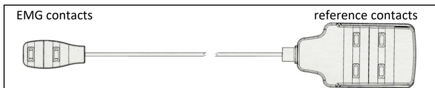
Figure 6. The EMG sensor head must be positioned overtop of the muscle of interest. The reference contacts can be positioned in a convenient nearby location.
