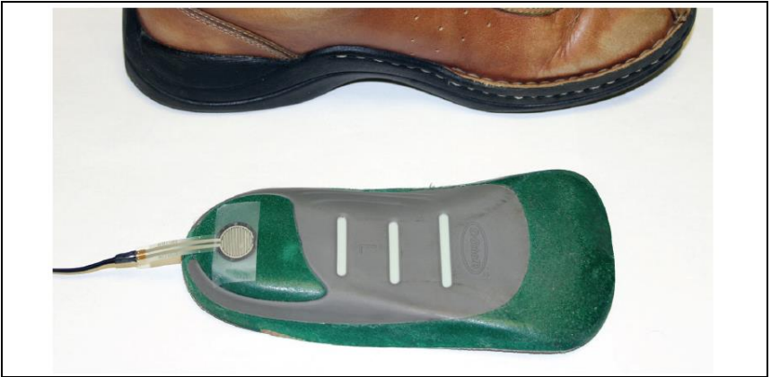
Figure 5: Affixing the FSR membrane to the bottom of the inner sole.
