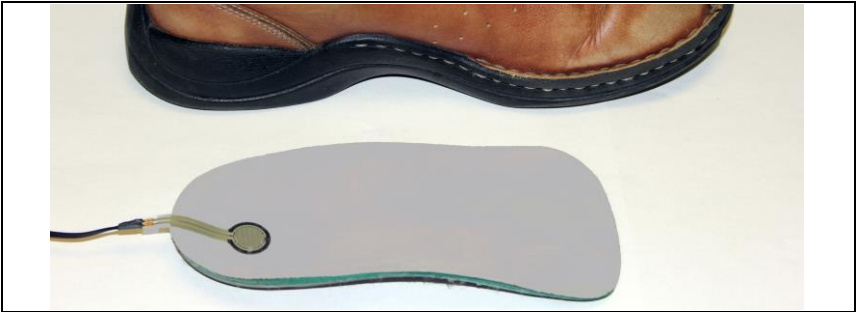
Figure 4: Affixing the FSR membrane to the top of the inner sole.
