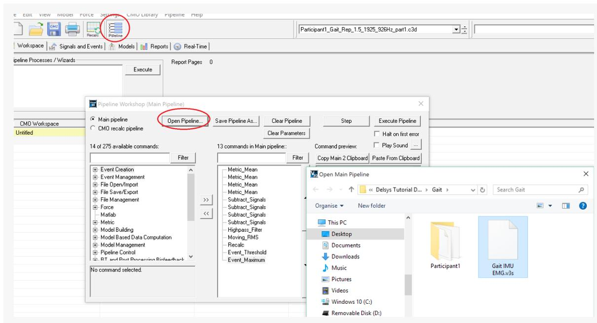
Figure 15: a) Opening and Running a pipeline in Visual3D
