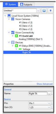
Figure 21: Configuring Delsys EMG channel settings in Vicon Nexus.
