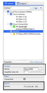
Figure 18: Adding in the Lock+/Lab Source in Vicon Nexus.
