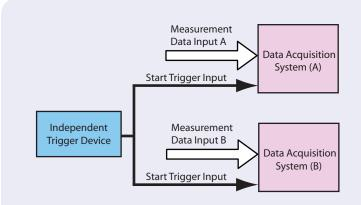
Figure 4: All data acquisition systems are started by an independent device that issues a common Start Trigger Input.
