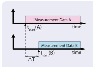
Figure 1: It is important to ensure that the time delay in starting multiple data acquisition system is minimized to an acceptable period.
