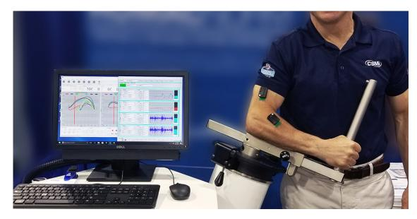
Delsys, Inc. will be attending the **ISB 2017 Conference** next week in **Brisbane**, **QLD**. We'll be showcasing our new **Trigno™ Avanti Sensor**, an advanced EMG/IMU sensor with the ability to communicate directly to tablets via Bluetooth or Trigno base stations via proprietary RF protocol.
